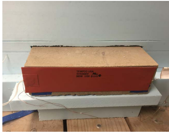
Figure 3-8: Flexible strip heater on exterior side of CSEB
