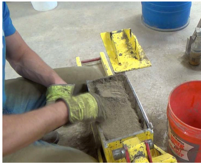
Figure 3-2: Tamping the soil-cement mixture into the block press
