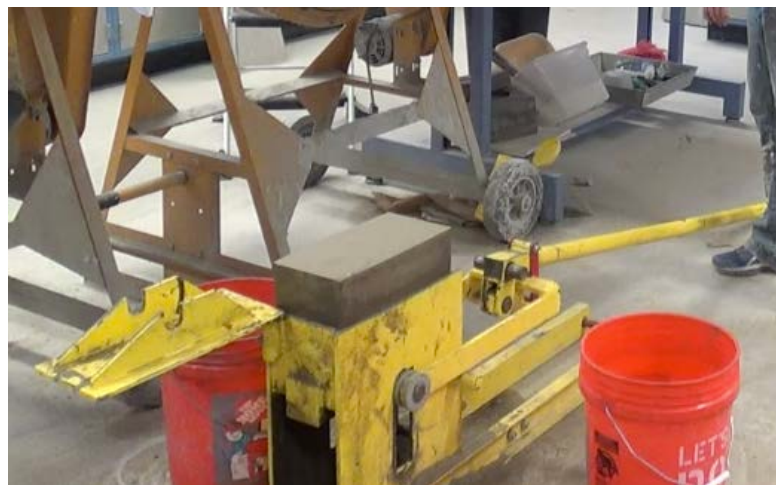
Figure 3-3: Finished CSEB after block press
